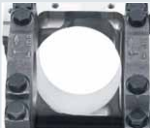
Top—Splayed Main Cap C Bottom—Machined Bottom (close-up)
