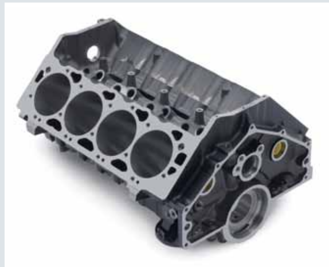
A 502 Mark IV/Gen VI Bare Block (rear)
