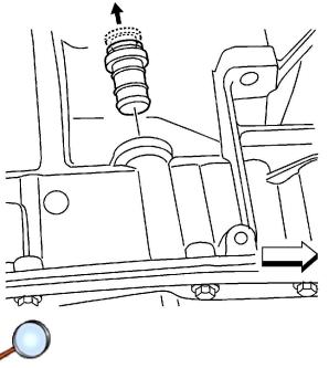
1. It may be necessary to use a long pair of 90 degree needle nose pliers to lift the plunger and remove the plug assembly.
