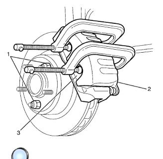
4. Install two wheel nuts (1) in reverse to opposite wheel studs to retain the brake disc to the hub.
