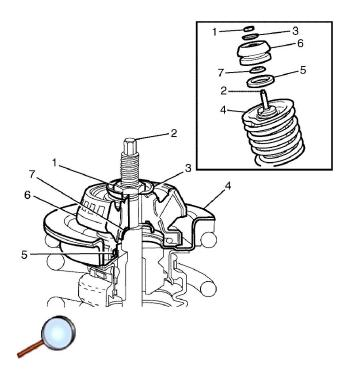
Important: The front strut assembly support bearing (5) is a sealed part and is replaced as an assembly.
