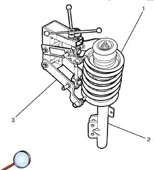
Caution: Use only the CH-48845 Spring Compressor when servicing suspension components on this vehicle. Other tools may not be strong enough for the springs on this vehicle and you could be injured if you do not use Special Tool CH-48845. Failure to do so could result in serious personal injury.
