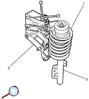
6. Make sure that the coil spring (1) is correctly positioned to the front strut assembly (2).
