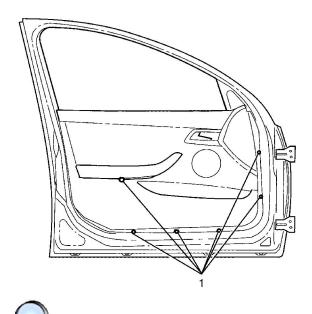
5. Install the door trim panel to door retaining screws (1).
