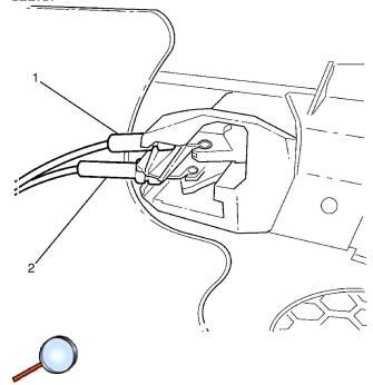
**Important:** The door handle and lock cables slide out and lift up to remove from the door trim panel.
