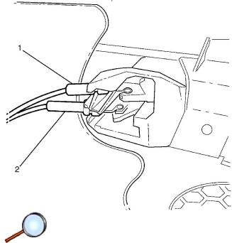
**Important:** The door handle and lock cables slide down and in to the door trim panel to install.
