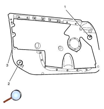
**Important:** Datum pins (1, 2) assist in aligning the door trim panel to the door.
