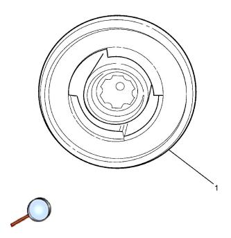
**Important:** Ensure the adjustment shaft is engaged in the sleeve.
