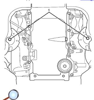
25. Remove the lower engine mount to crossmember retaining nut (1) from both engine mounts.
