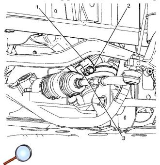
Note: The intermediate steering shaft and pinion shaft splines must be installed in the position recorded during removal and aligned with the marks previously made.
