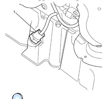
16. Disconnect the oil level/temperature sensor electrical connector (1) from the oil level/temperature sensor.
