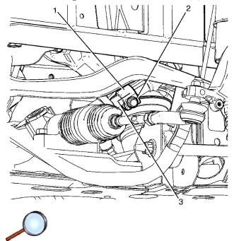
**Note:** Observing the orientation of the intermediate steering shaft (1) with reference to the pinion shaft (3) will minimize the potential of incorrect steering column assembly alignment.
