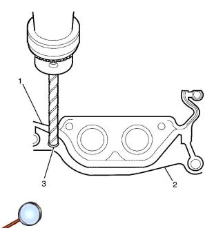
**Note:** DO NOT allow foreign material to enter the oil passages of the oil pan, cap, or cover the openings, as required.
