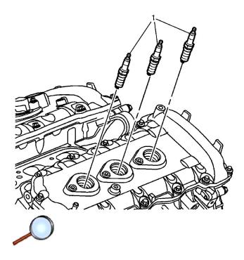
**Caution:** Use only the spark plugs specified for use in the vehicle. Do not install spark plugs that are either hotter or colder than those specified for the vehicle. Installing spark plugs of another type can severely damage the engine.
